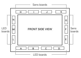
2. When all components of test board D (LED) and all components of test board K (Sens) are malfunctioning. The detailed list indicates "ALL" and not data for each Point.
